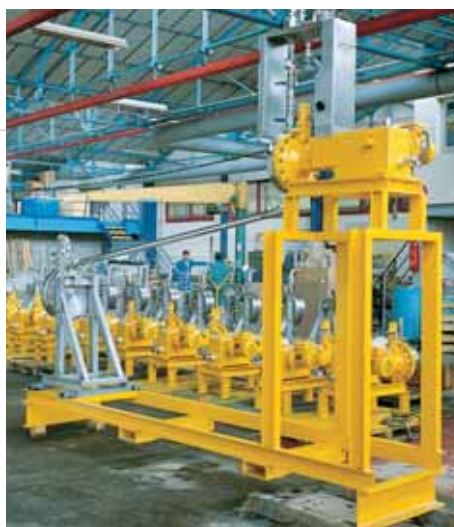
Dosing aqueous and organic phases in uranium enrichment.
