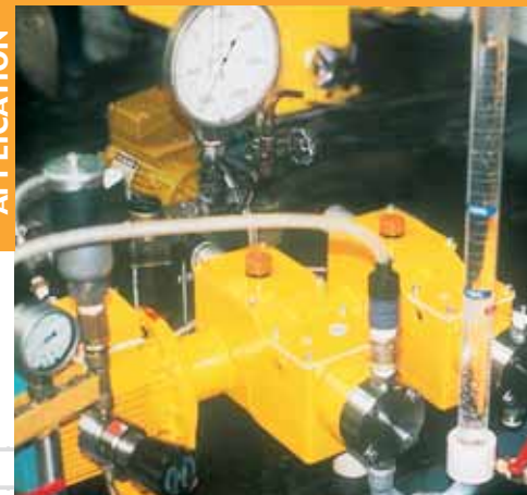
Sample being taken in an extraction column at high vacuum (7 torr).
